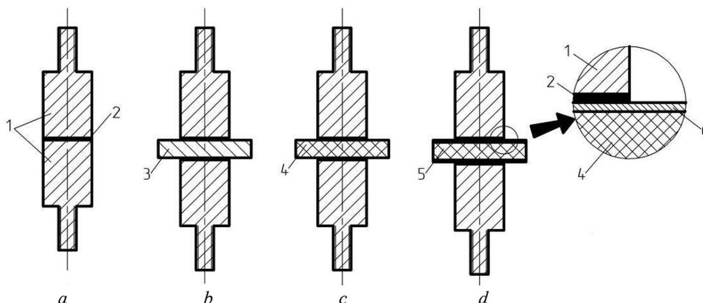
Fig. 4. Variants of gluing materials for establishing adhesive strength:
