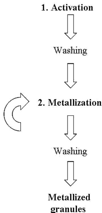
Fig. 1. Scheme of production of copper-plated polyamide granules
