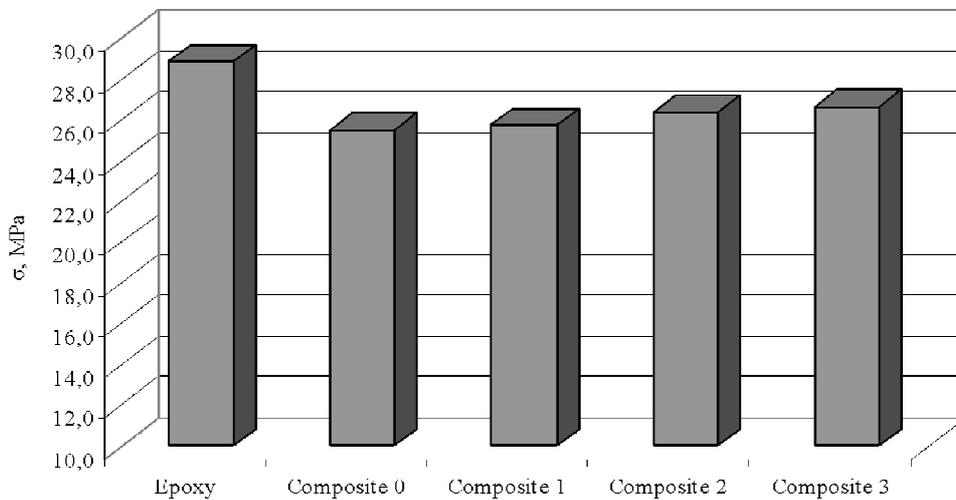
Fig. 8. Tensile strength of composites with an epoxy matrix
