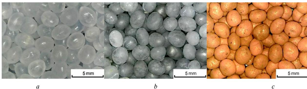
Fig. 5. Photographs of initial (*a*), activated (*b*) and copper-plated polyamide granules (*c*)
