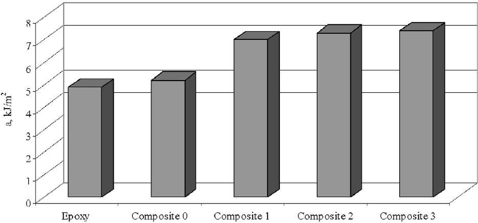
Fig. 9. Impact toughness of composites with an epoxy matrix
