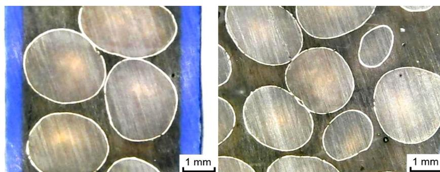
*Fig. 3. Distribution of copper-plated granules in the epoxy matrix (the photos were obtained after grinding the samples and the copper shell is visible on them)*
