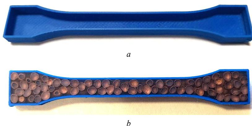
*Fig. 2. An example of a form obtained by 3D printing for forming a sample intended for tensile strength studies (a) and a sample prepared for studies (b)*
