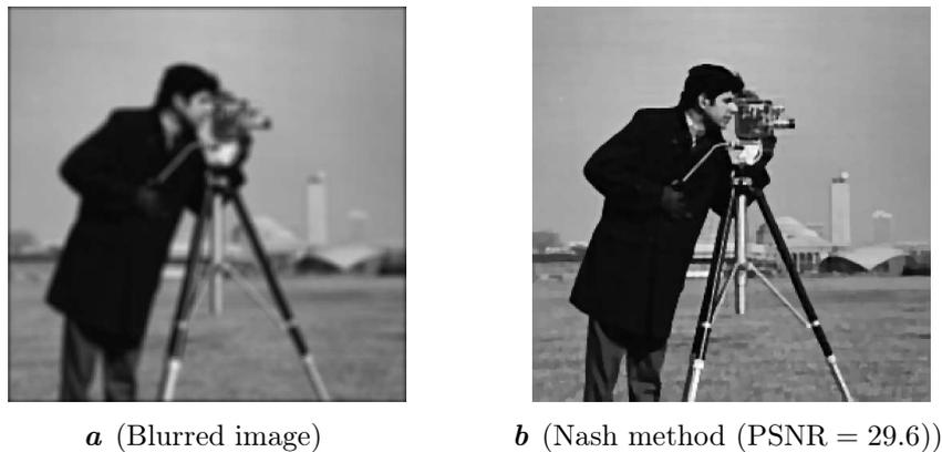
**Fig. 2.** The Nash method experiment on the Cameraman image.
