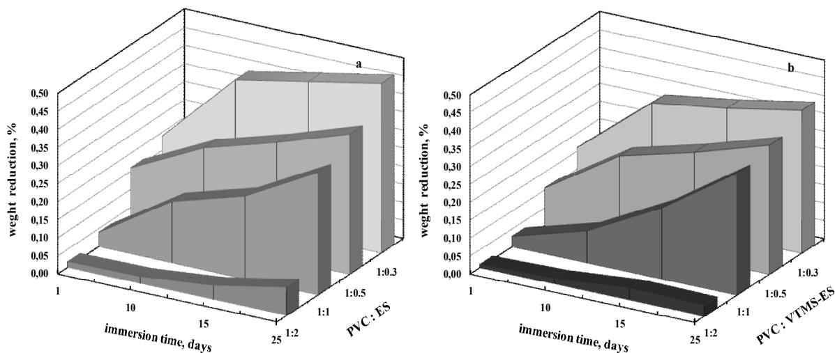
**Fig. 1.** Weight reduction of PVC films with different ratios of untreated (a) and silane-treated (b) eggshell fillers after immersion in water
