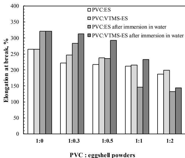
**Fig. 3.** Dependence of the elongation at break of PVC films with different ratios of untreated and silane-treated eggshell fillers before and after immersion in water
