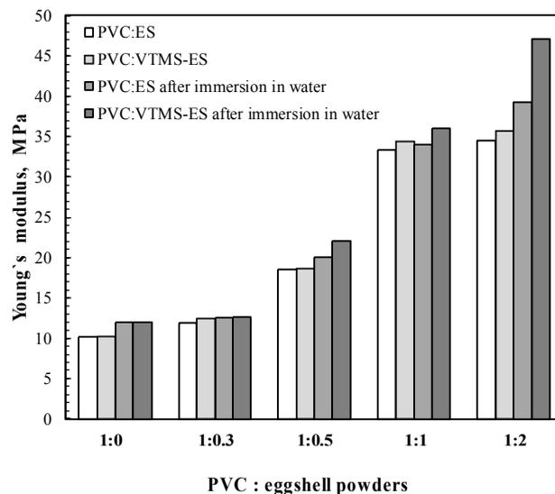
**Fig. 4.** Dependence of the *Young's* modulus of PVC films with different ratios of untreated and silane-treated eggshell fillers before and after immersion in water
