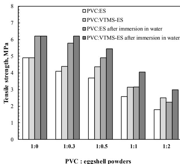
**Fig. 2.** Dependence of the tensile strength of PVC films with different ratios of untreated and silane-treated eggshell fillers before and after immersion in water
