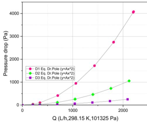
**Fig. 4.** Graphical representation of the pressure drop vs. the air flow rate at standard conditions, for the three copper pipes
