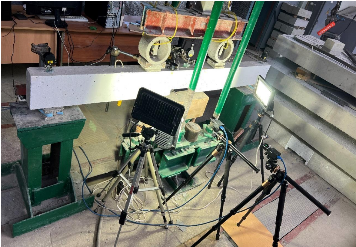
Fig. 7. Overall view of the camera arrangement for image capture
