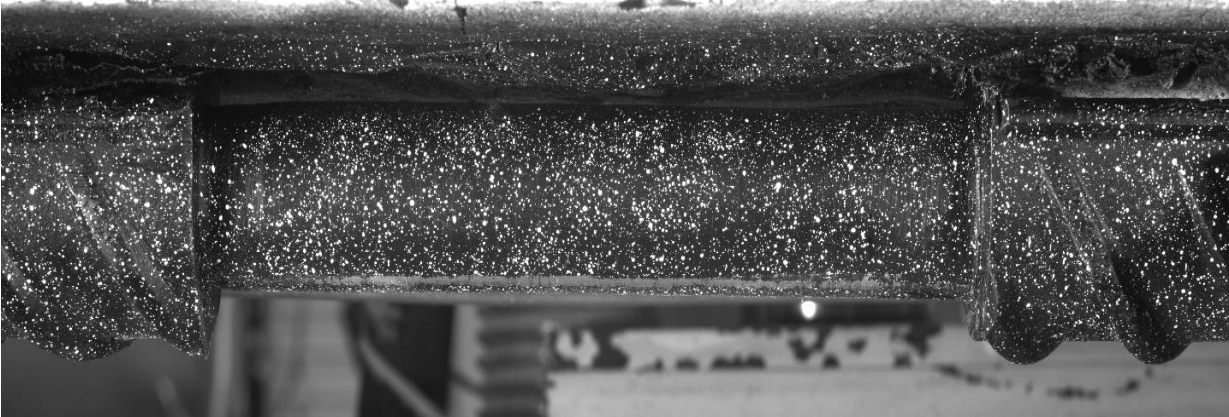
Fig. 6. Applied speckles on reinforcement
