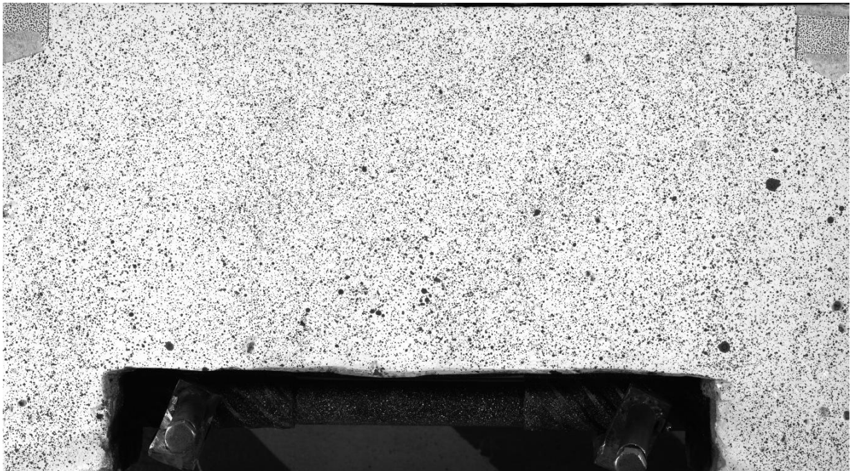
Fig. 5. Applied speckles on concrete
